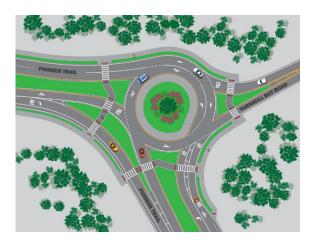
Roundabouts also significantly reduce the number and complexity of conflict points between vehicles, substantially lowering the risk of serious injuries or fatalities. Additionally, the slower speeds at roundabouts further reduce the severity of crashes.
