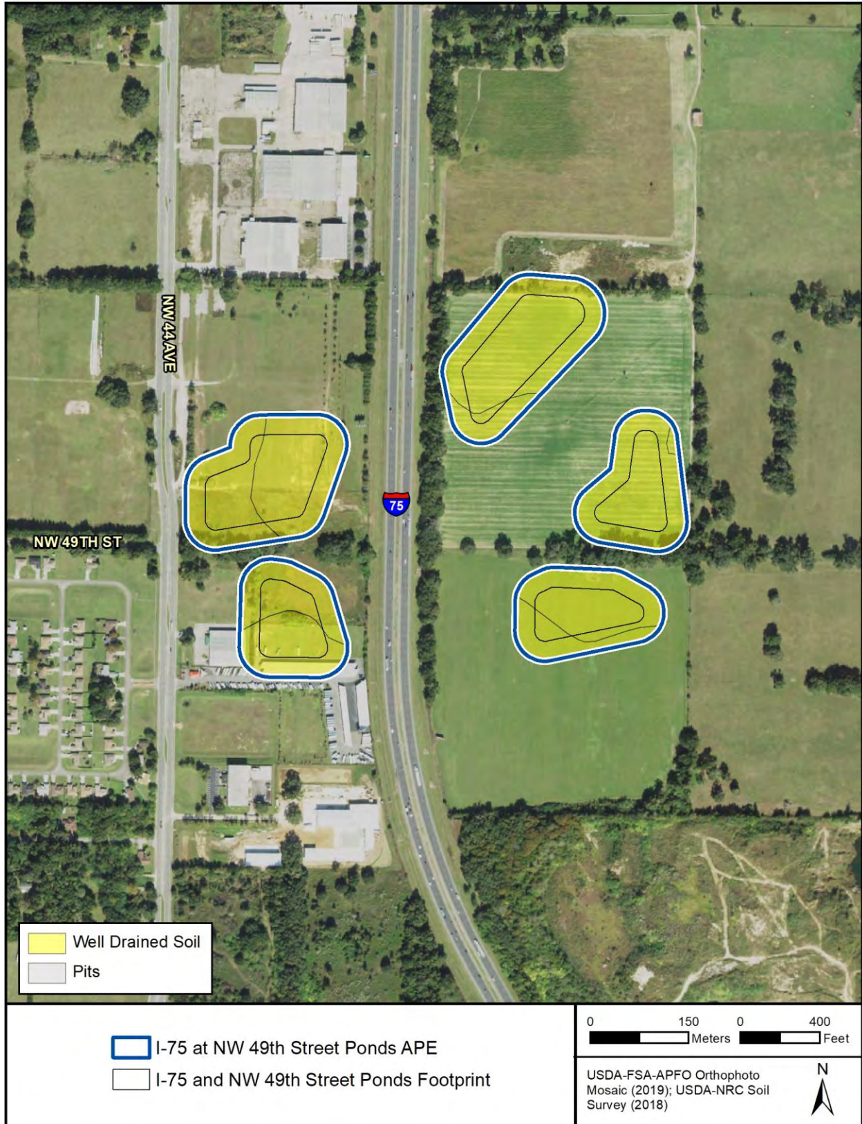
Figure 4. Soil drainage characteristics within the I-75 at NW 49th Street Ponds APE.
