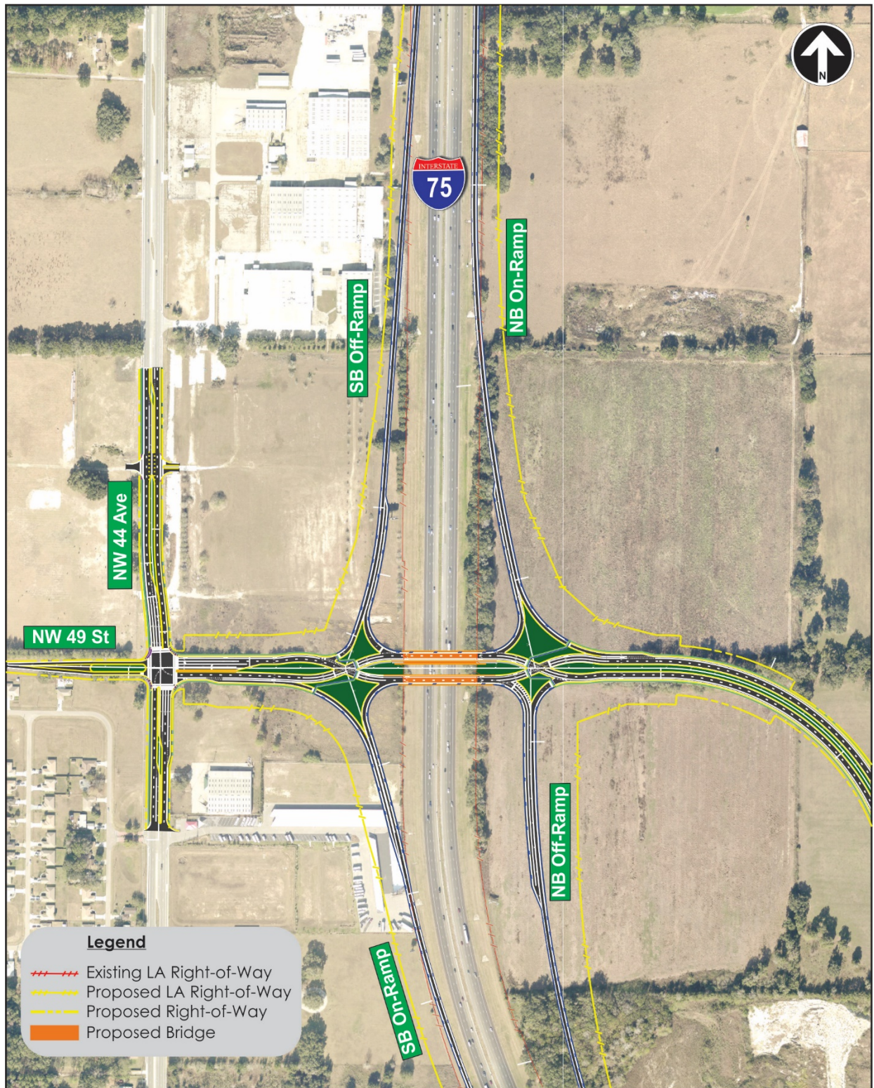
Figure 4-6 - Preliminary Diverging Diamond Interchange
