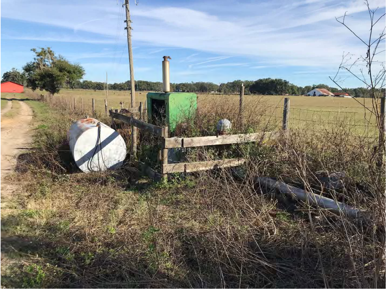
Aboveground Storage Tank, Outside Project Area, Likely Fuel for Irrigation Pump
