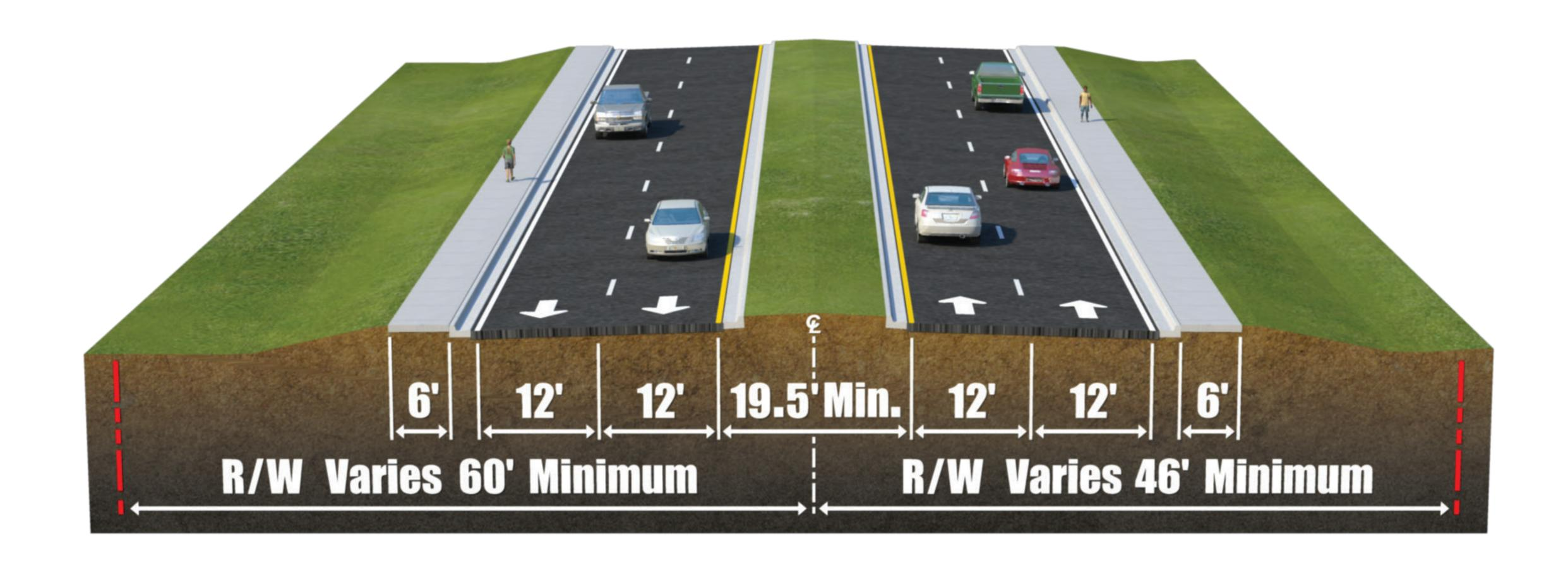
NW 44th Avenue Proposed Typical Section Design Speed: 45 mph
