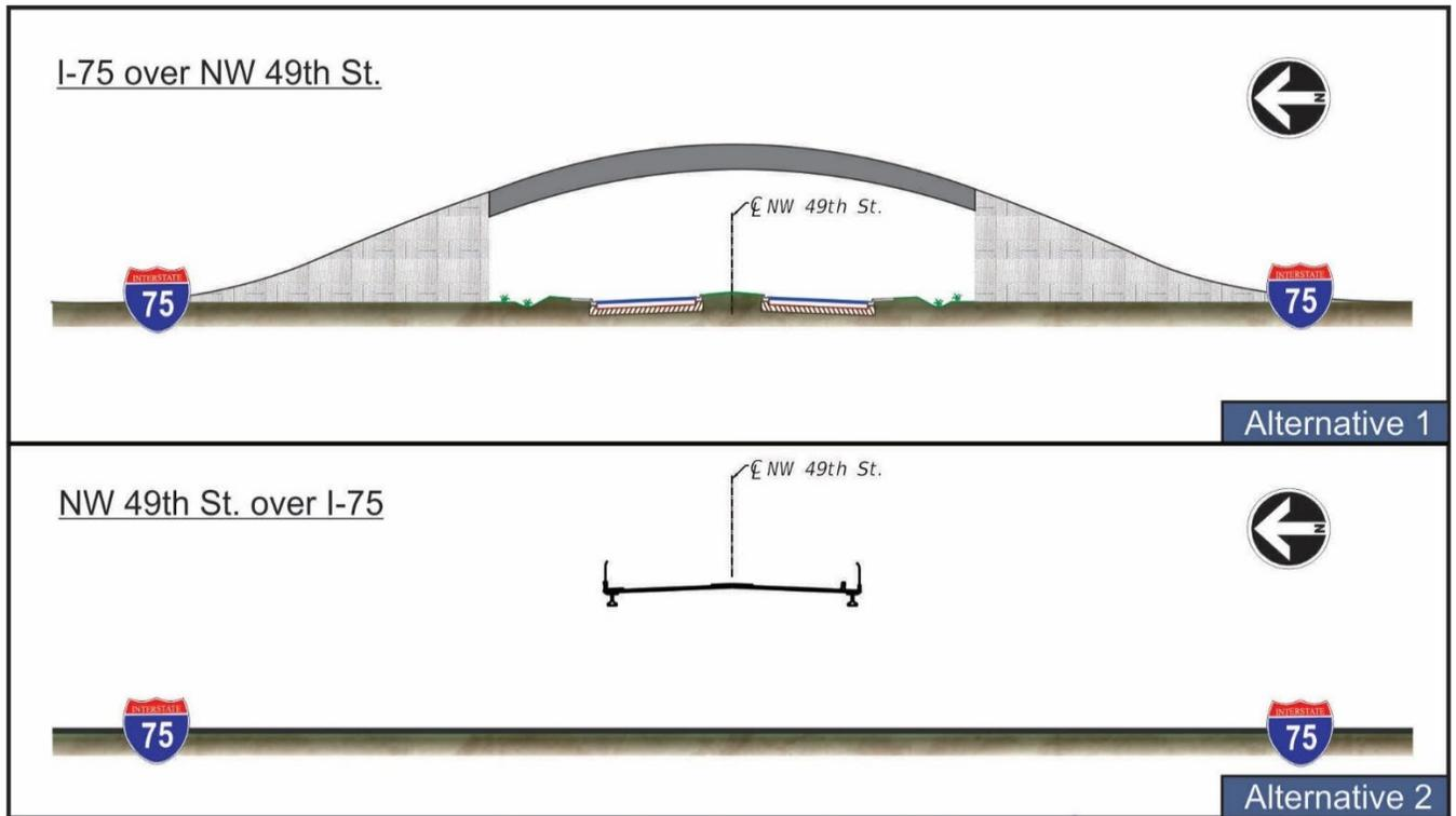
Figure 3- Alternatives 1 and 2 – Plan and Profile
