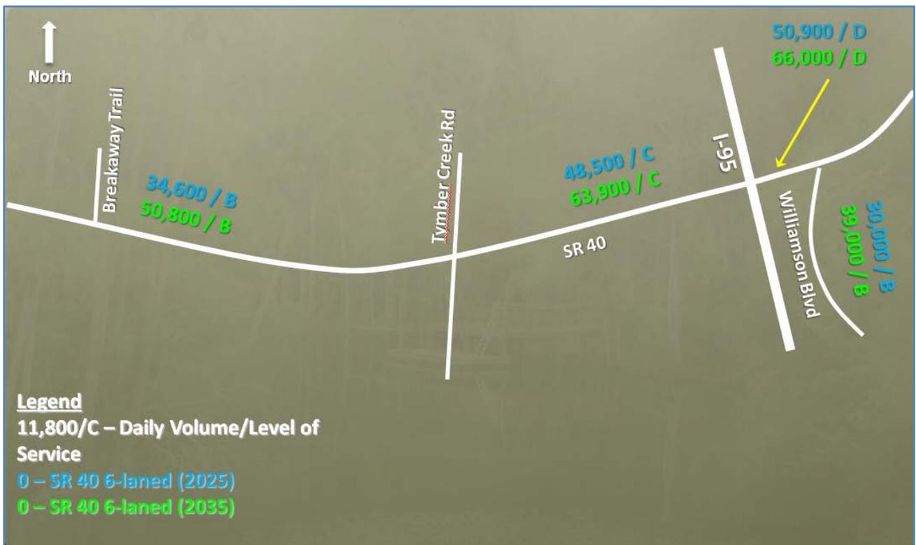
Figure 3-2 Build Alternative 5 AADT Volumes and Level of Service
