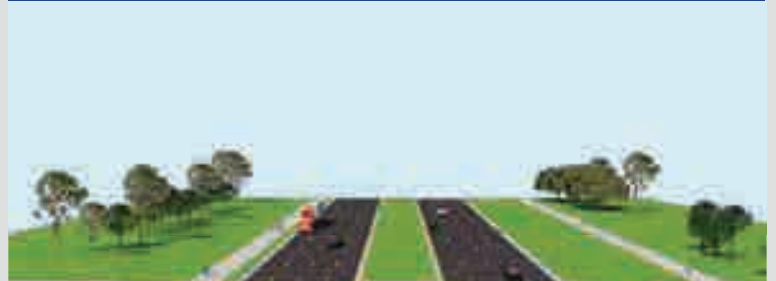
Eight lanes with divided median
