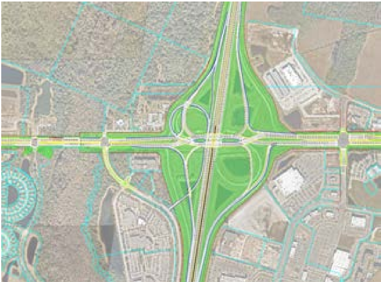
Figure 4.7 | Diverging Diamond Interchange
