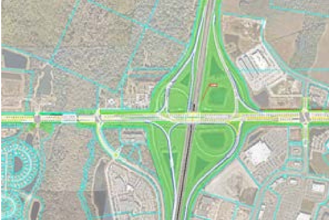
Figure 4.11 | Displaced Left Diamond Interchange
