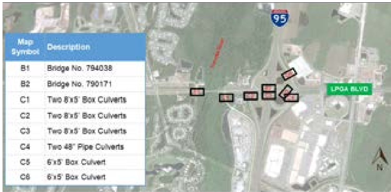
Figure 2.5 | Existing Structure Locations and Summary Information
