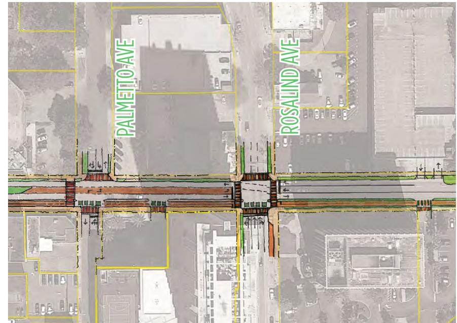
The three-lane cross section with two-way cycle track on the south side of the street would be carried through Rosalind Avenue to the Lake Eola District.
