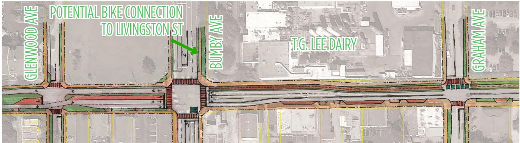
The two-way cycle track would be re-introduced on the north side of Robinson Street at Bumby Avenue, and permanent on-street parking spaces would be added on the south side, where possible, to support the businesses in this area.
