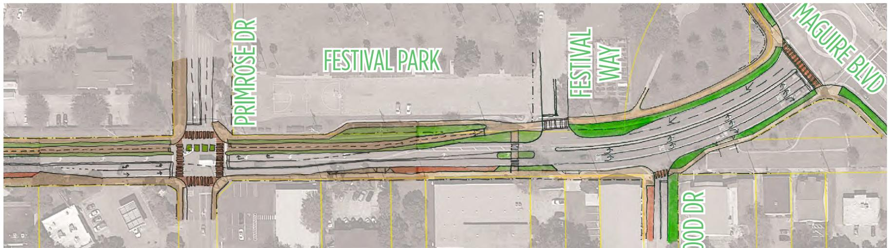
On the eastern end of the corridor, the two-way cycle track would transition to a wide sidewalk just west of Maguire Boulevard, and eventually connect to the shared use path that runs along the east side of Maguire Boulevard.
