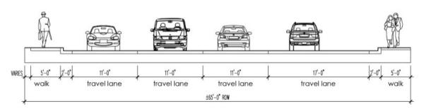
Figure 12: White Street Typical Cross Section
