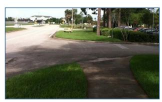
A non ADA compliant bus stop and sidewalk gap on Richard Petty Blvd at Corsair Dr. The bus stop is located on the utility pole above the bench in the background.
