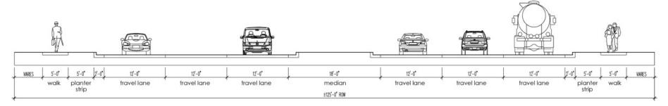
Figure 5: SR 5A/Nova Road Typical Cross Section
