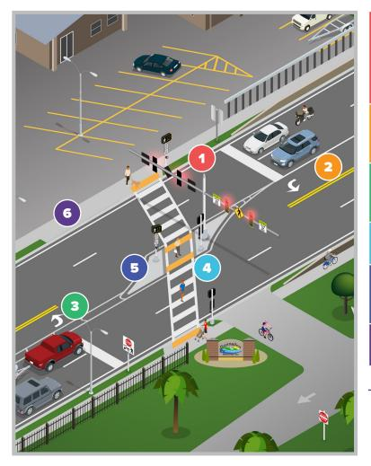
A new Midblock Pedestrian Signal allows pedestrians to cross safely by pushing a button to stop traffic. Motorists will see the red light and must stop. The light then changes to a flashing red which allows traffic flow if pedestrians have crossed.
