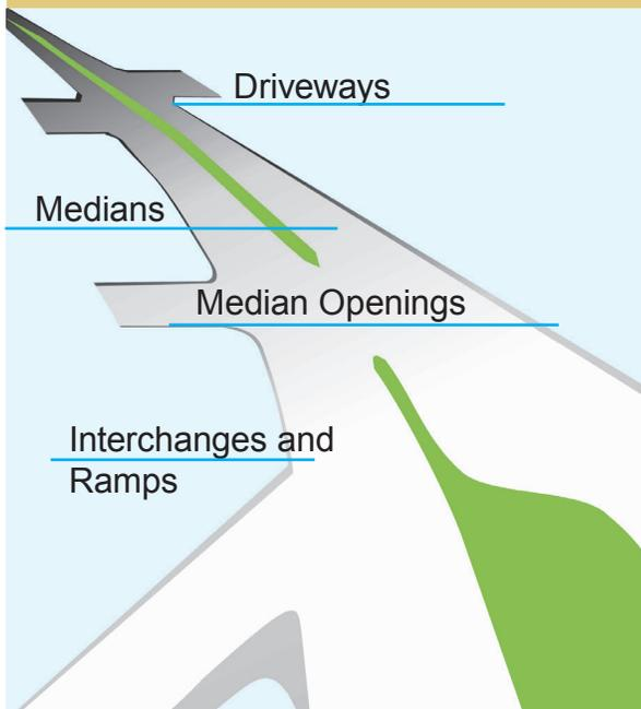
The purpose of access management is to provide access to land development in a manner that preserves the safety and efficiency of the transportation system.
