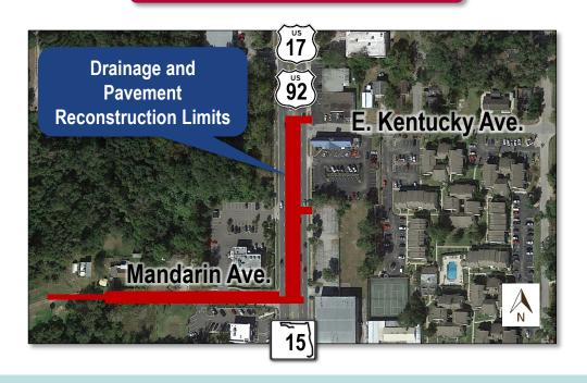
The Florida Department of Transportation (FDOT) is proposing drainage improvements on North Woodland Boulevard from Mandarin Avenue to north of East Kentucky Avenue. Proposed improvements consist of adding drainage inlets, adding underground drainage pipes along the median of North Woodland Boulevard and Mandarin Avenue, relocating utilities, and repaving North Woodland Boulevard and Mandarin Avenue within the project limits.
