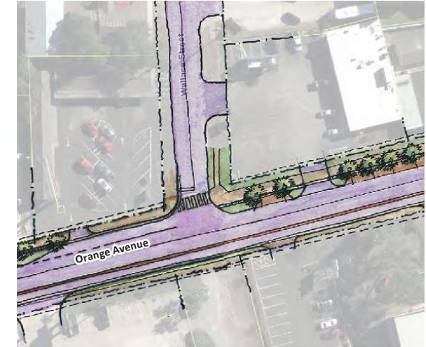
**Figure 64 | Potential Driveway Consolidation/ Refinements along the Corridor (Example along the Corridor at Wallace Street)**
