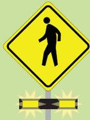
The yellow lights begin flashing rapidly indicating to motorists that a pedestrian is attempting to cross, and that the motorist must stop or clear the crossing, if they are too close to stop. The beacon continues flashing for a time appropriate to the crossing distance. Motorists must continue to remain stopped until crossing pedestrians have cleared their lane, at which time they may proceed.
