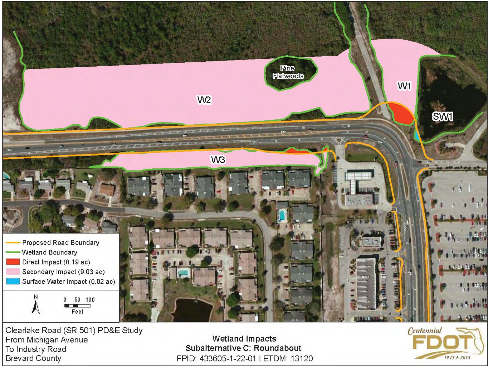
FIGURE 2(c): SUBALTERNATIVE C – ROUNDABOUT
