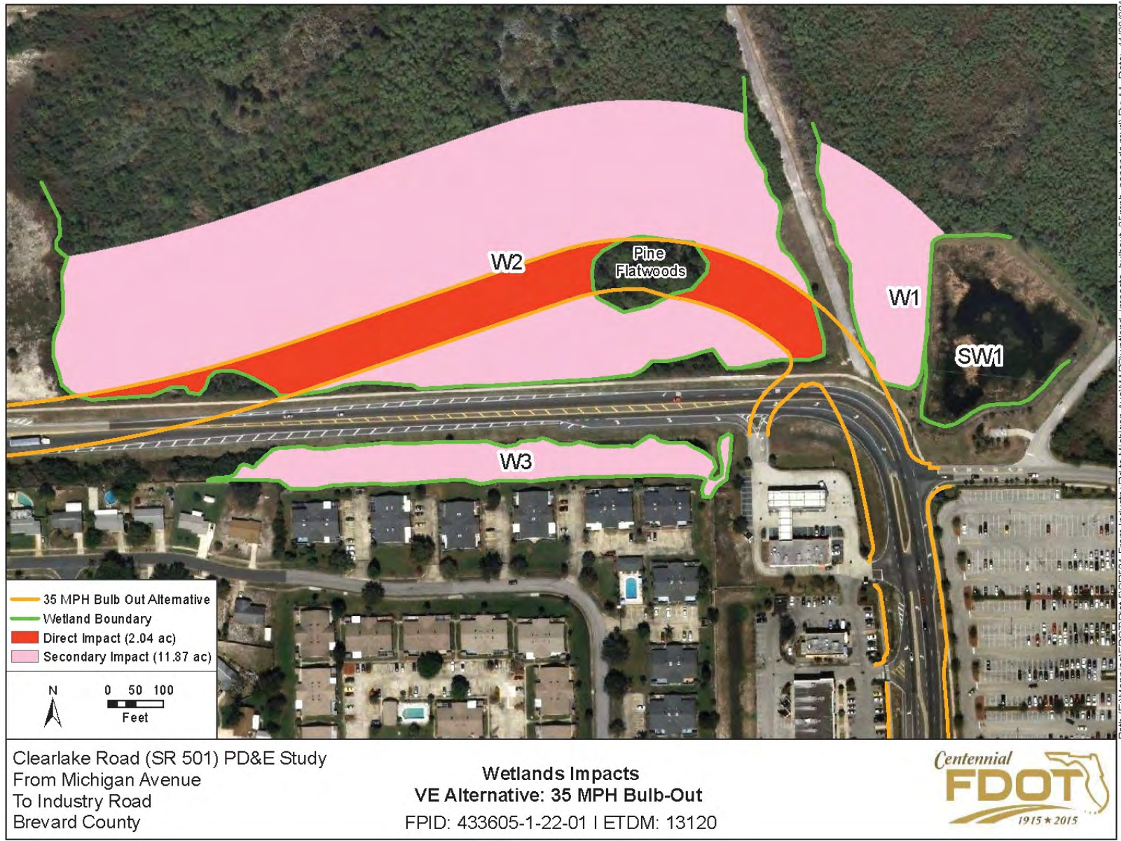
FIGURE 2(e): SUBALTERNATIVE – 35 MPH ‘BULB-OUT’
