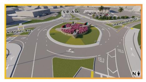
The proposed modern roundabout has two through lanes and one circulating lane, while the Viera roundabout has two circulating lanes. This additional circulating lane can create confusion over which lane drivers need to be in to make a turn. The roundabout in Cape Canaveral will not have this extra lane, making navigation much simpler.
