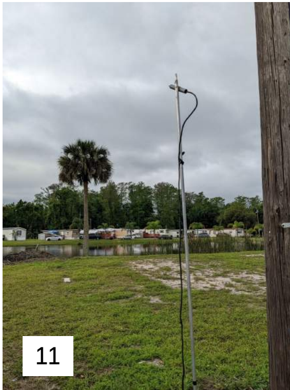
Photographs 11 and 12: View of Detector 6, illustrating the microphone was tilted vertically at approximately 45° (Photograph 11). View of the pond targeted at Detector 6 (Photograph 12).
