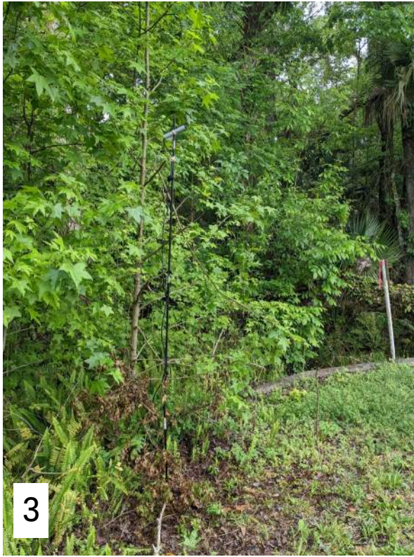
Photographs 3 and 4: View of Detector 2, illustrating the microphone was tilted vertically at approximately 45° (Photograph 3). View of the location targeting commuting bats traveling along the wetland forest edge and road corridor (Photograph 4).
