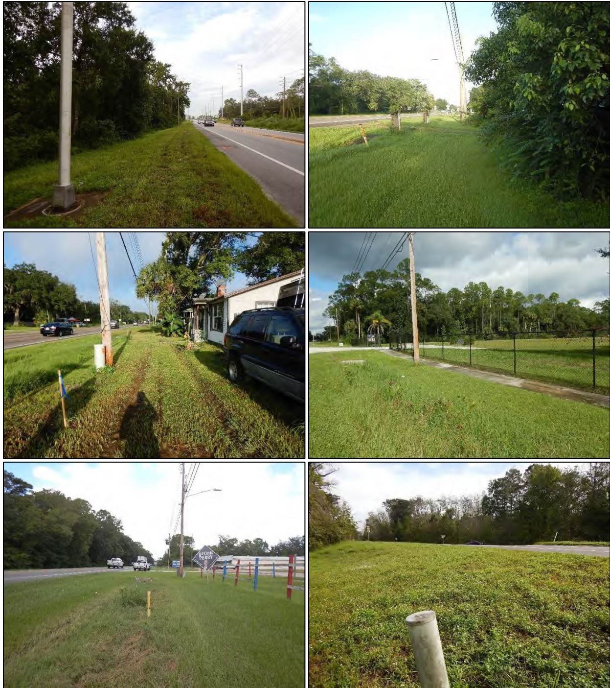
Figure 17. Representative views of existing disturbances within the US 17/92 Right-of-Way. Top left: Lighting pole, fiber optic cable locate markings, and raised roadbed at Shovel Test 28, facing south. Top right: Gas line marker and drainage system at Shovel Test 76, facing west. Center left: Utility pedestal, overhead electric, and drainage ditch at Shovel Test 78, facing west. Center right: Overhead electric, drainage ditch, and existing sidewalk at Shovel Test 84, facing north. Bottom left: Gas line, overhead electric, and drainage ditch at Shovel Test 85, facing west. Bottom right: Utility pedestal and raised roadbed at Shovel Test 89, facing east.
