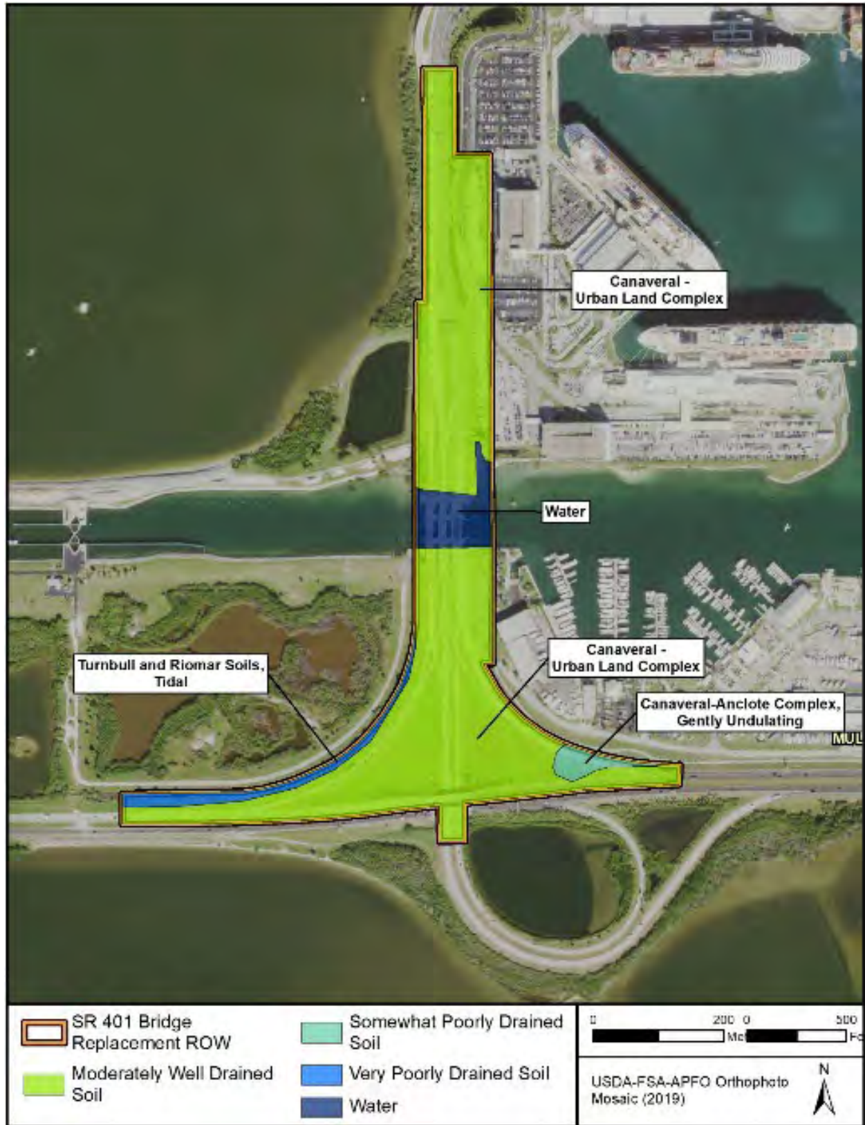
Figure 3. Soil types and drainage within the SR 401 Bridge Replacement right-of-way.
