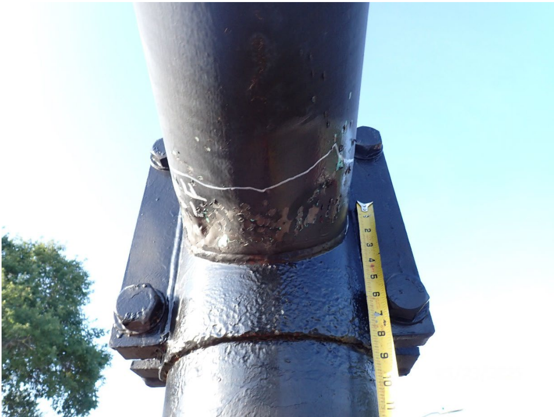
Photo 2: V2/H2 – Malleable area on underside of arm
