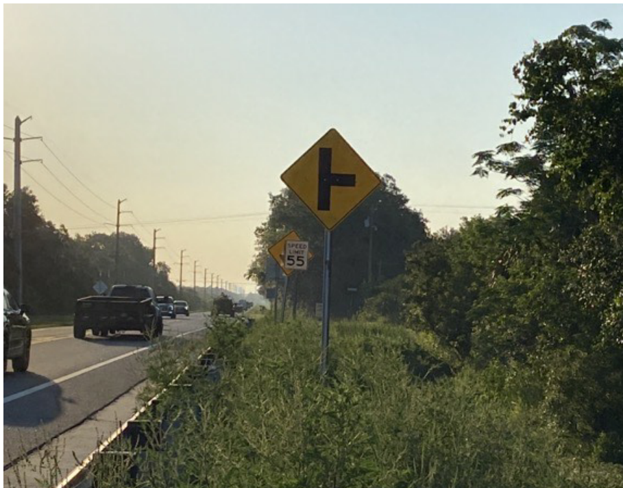
Figure 4-7 Two-way Traffic Sign Obstructed by Speed Limit Sign on Eastbound SR 46
