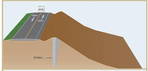
The northern most segment will include the construction of a seawall to protect the roadway. The wall will be buried by additional sand and dune plantings. An erosion control mat will also be installed to aid in sand and dune stabilization. A shallow swale will be constructed between the roadway and dune to help control water runoff. The project also will include milling and resurfacing of the roadway. Parking will be prohibited on the east side of the roadway to protect the dunes.
