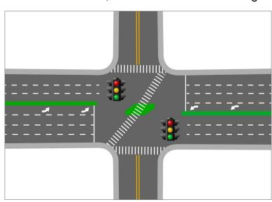
Operational and safety improvement proposed at Michigan Avenue include reconstructing and upgrading the existing traffic signal. New pedestrian signals and crosswalks will be installed at all intersections and lighting will be upgraded to enhance pedestrian safety. The project also includes reconstructing pedestrian curb ramps in accordance with current Americans with Disabilities Act (ADA) standards.
