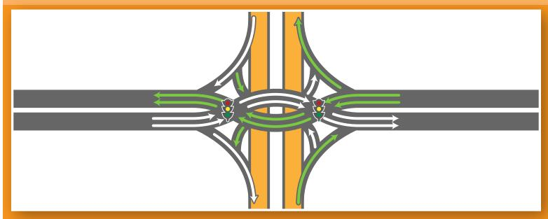
The diverging diamond interchange (DDI) eliminates left turn phases at traffic signals. It also reduces the number of traffic signal phases from four to two phases. The DDI will move almost double the traffic through the intersection in the same time.
