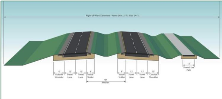
In addition, a new 250-foot long eastbound bridge will be constructed to match the existing bridge. The new bridge will be 56-feet wide, consisting of two 12-foot wide travel lanes and a 12-foot wide shared use path.
