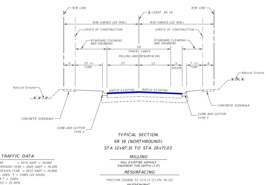
CURRENT YEAR ESTIMATED OPENING YEAR = 2020 AADT = 16,200 ESTIMATED DESIGN YEAR = 2022 AADT = 16,800 K = 9% D = 100% T = 3.68% (24 HOUR) DESIGN HOUR T = 3.68%DESIGN SPEED = 35 MPH POSTED SPEED = 35 MPH
