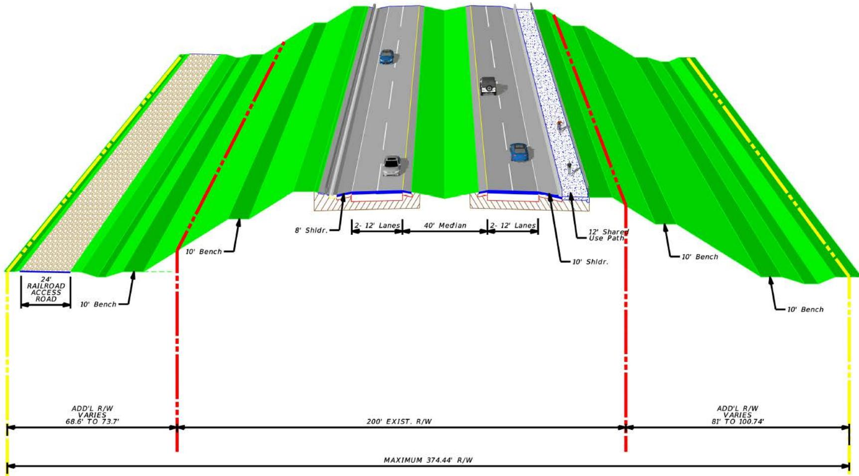
Figure 5: Typical Section – Hernando/Sumter County Line to Lee Road (Minimum ROW with Resurfacing Existing Roadway)
