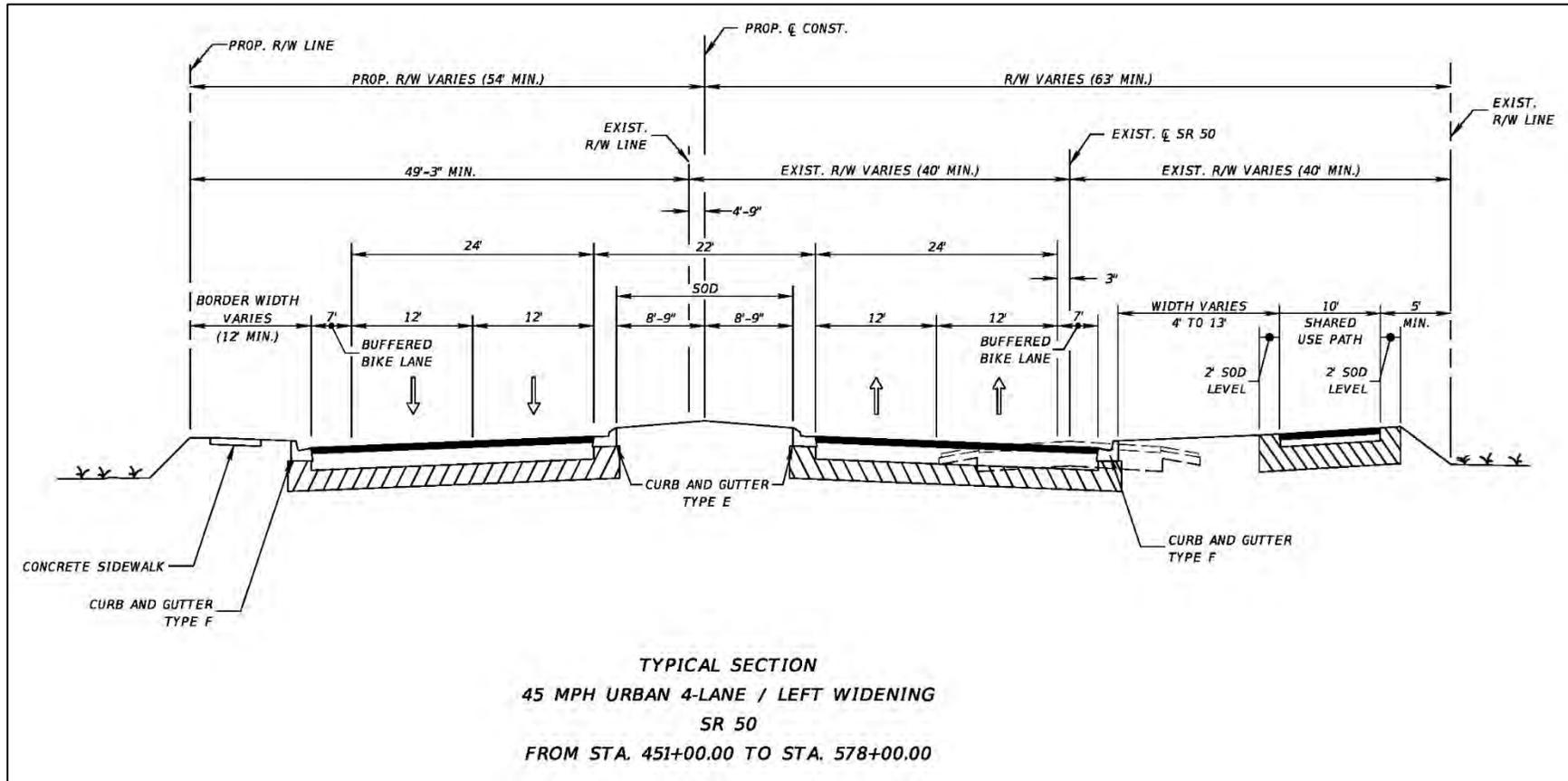
Figure 66: Urban Four-Lane Center Widening – Station 451+00 to Station 578+00
