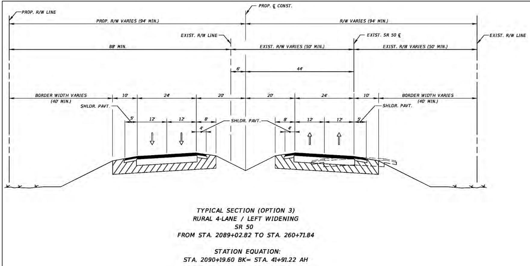
Figure 57: Rural Four-Lane Center Widening – Station 2089+02 to Station 260+71
