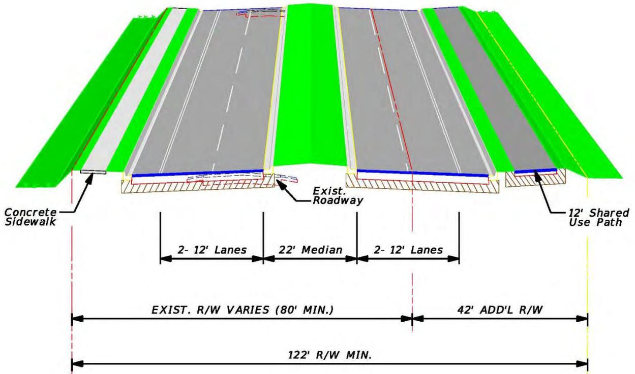
Figure 89: Typical Section – Lee Road to West of Barry Avenue (Maximum ROW with Drainage Conveyance Ditches)
