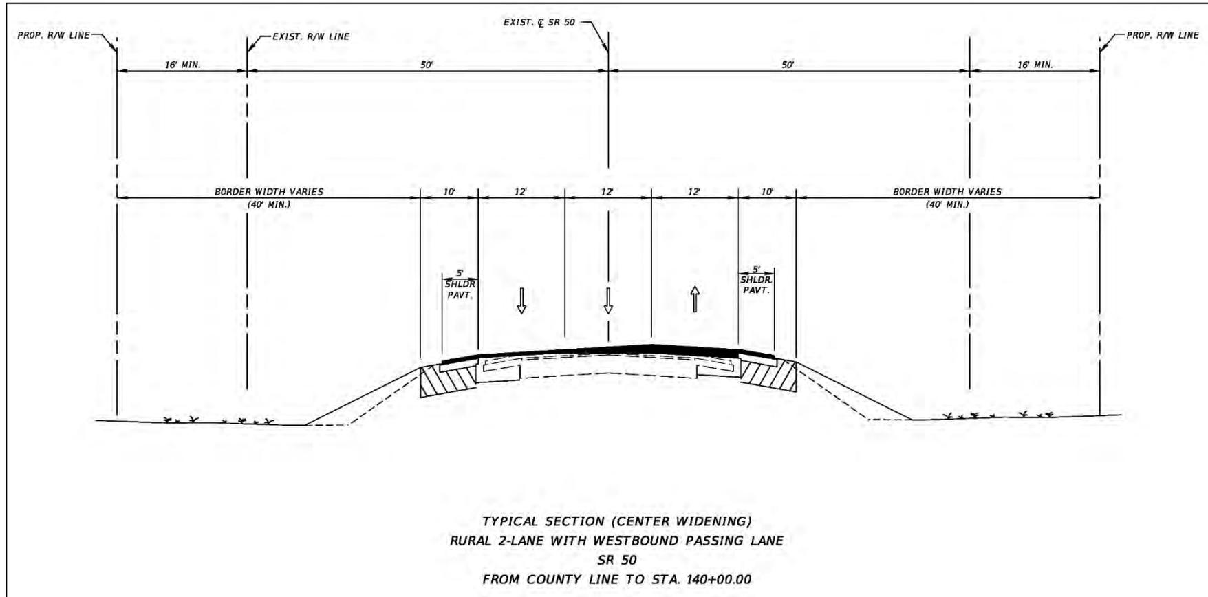
Figure 55: Westbound Passing Lane Right Widening – Station 2089+02 to Station 140+00
