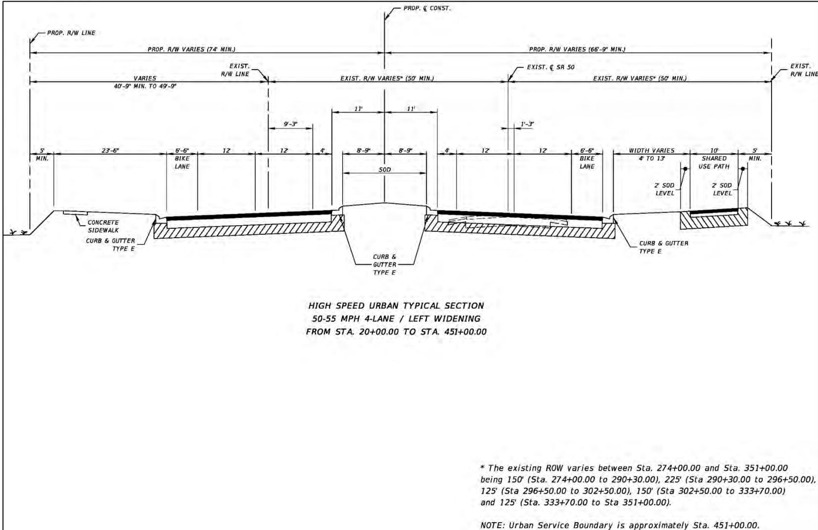
Figure 63: High Speed Urban Four-Lane Center Widening – Station 20+00 to Station 451+00
