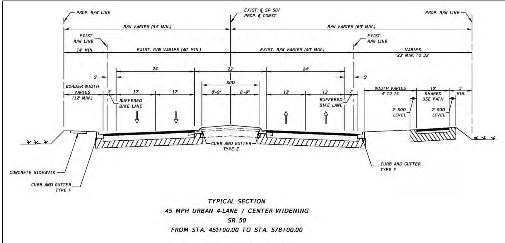
Figure 67: Urban Four-Lane Right Widening – Station 451+00 to Station 578+00
