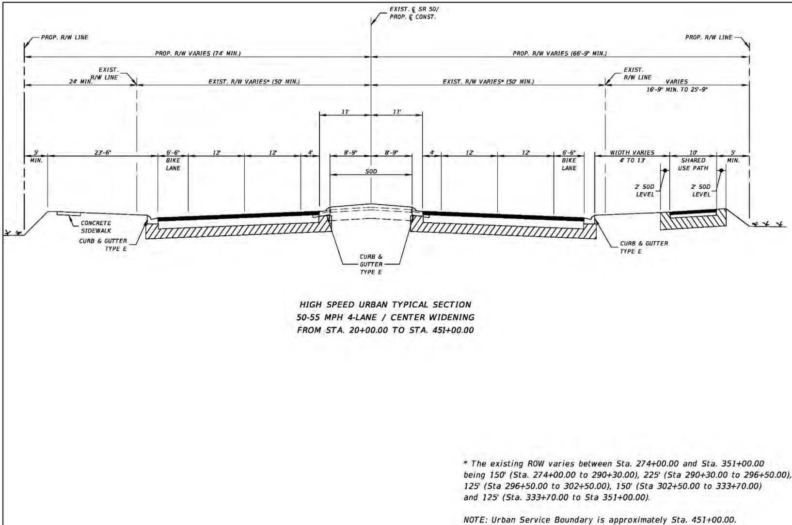
Figure 64: High Speed Urban Four-Lane Right Widening – Station 20+00 to Station 451+00
