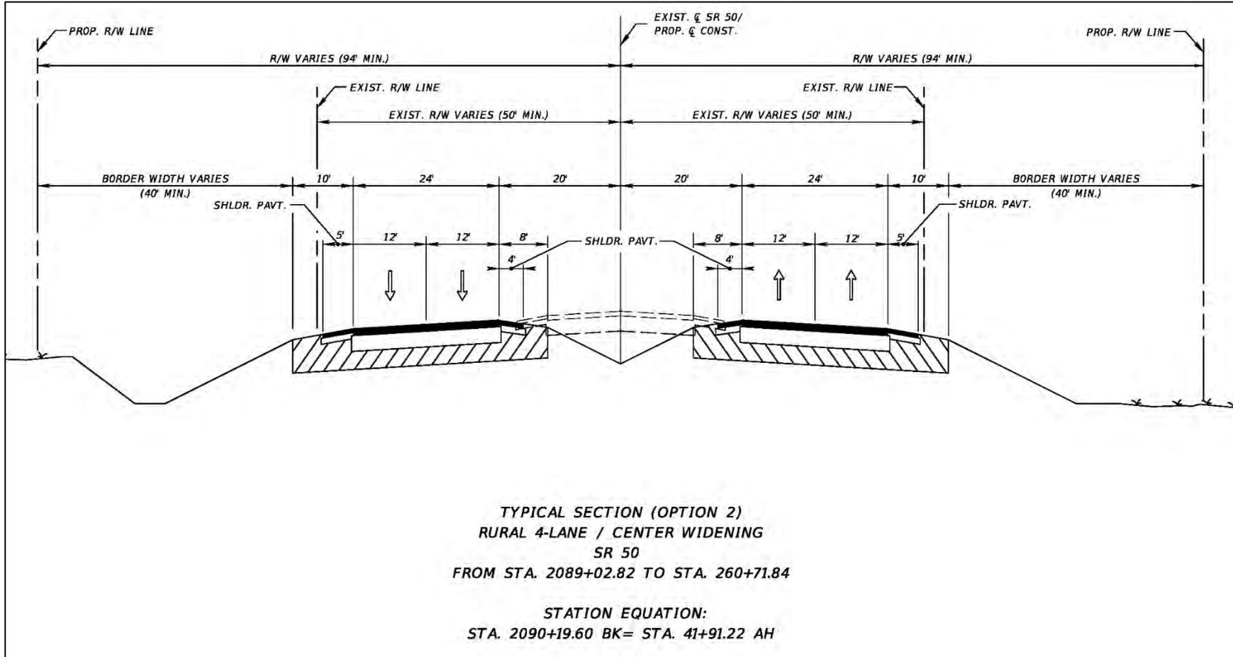
Figure 58: Rural Four-Lane Right Widening – Station 2089+02 to Station 260+71
