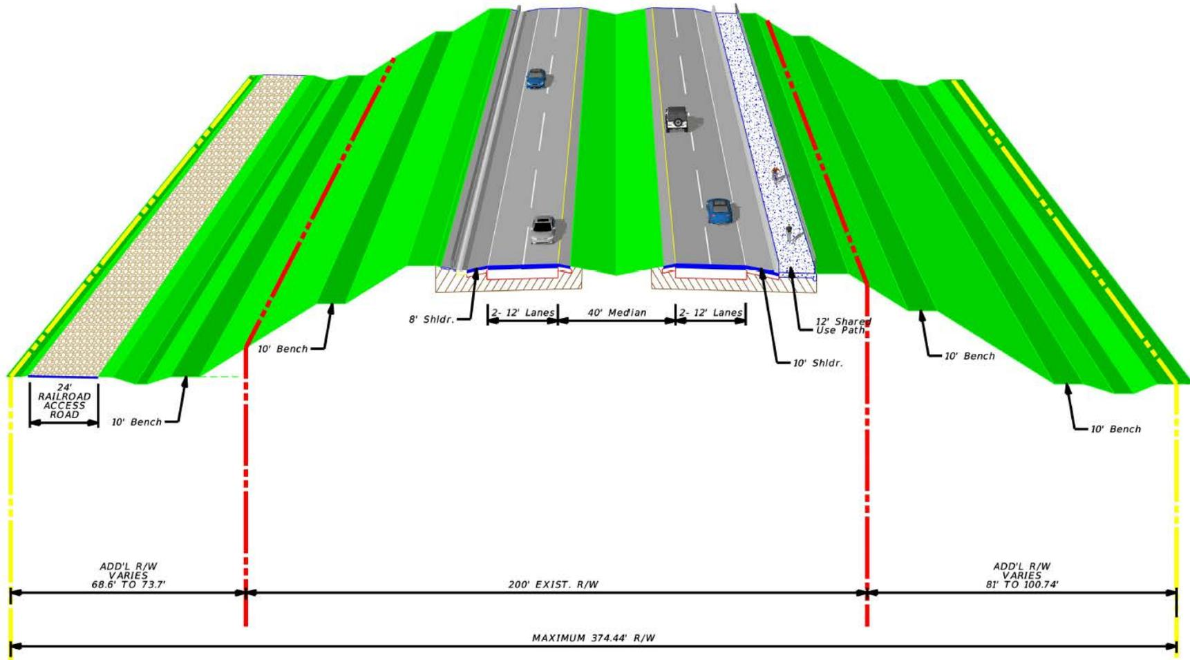
Figure 85: Typical Section – Hernando/Sumter County Line to Lee Road (Minimum ROW with Resurfacing Existing Roadway)
