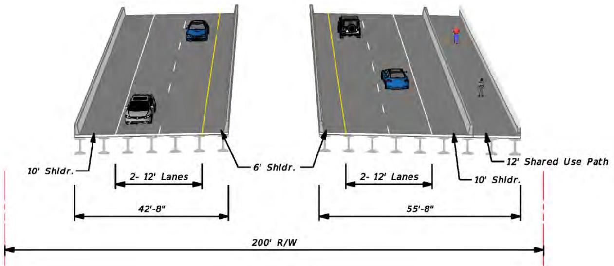
Figure 4: Typical Section – U.S. 301 to Hernando/Sumter County Line (Maximum ROW at Railroad Overpass Approach)
