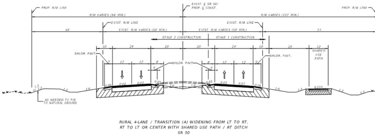
Figure 101: Rural Transitioning Widening Alternative
