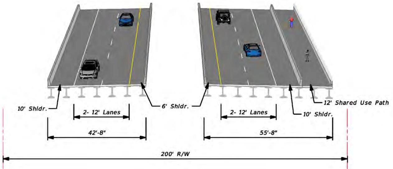
Figure 84: Typical Section – U.S. 301 to Hernando/Sumter County Line (Maximum ROW at Railroad Overpass Approach)
