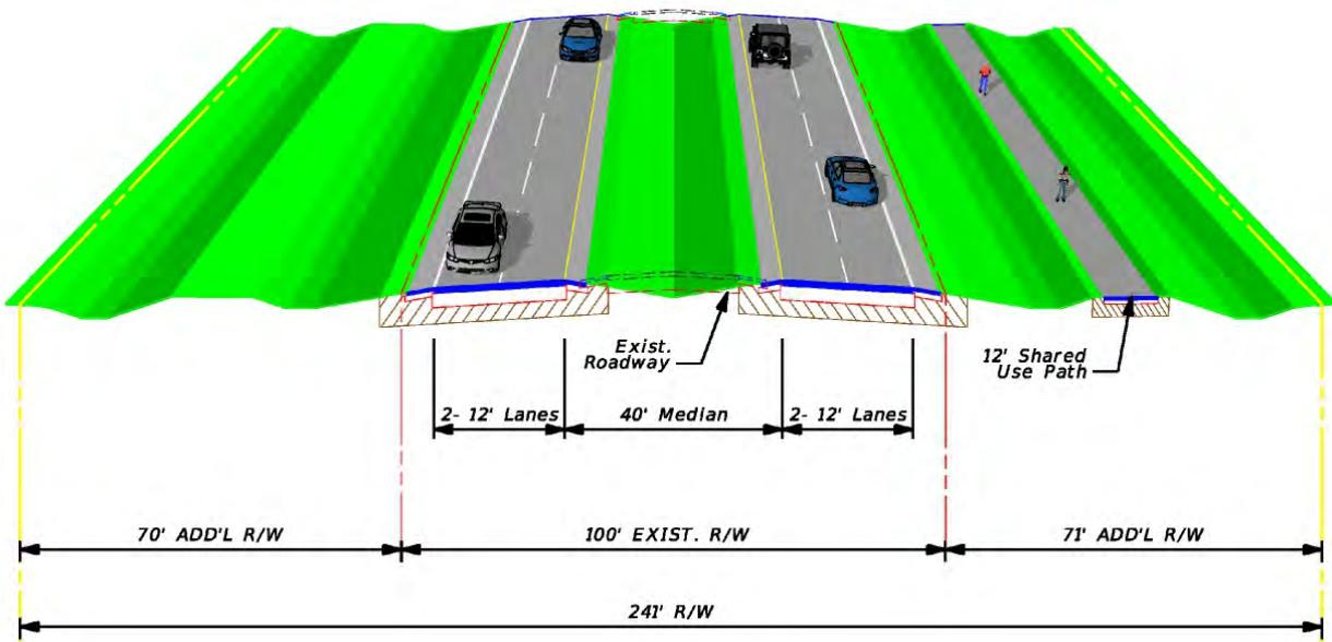
Figure 87: Typical Section – Hernando/Sumter County Line to Lee Road (Little Withlacoochee River Bridges)
