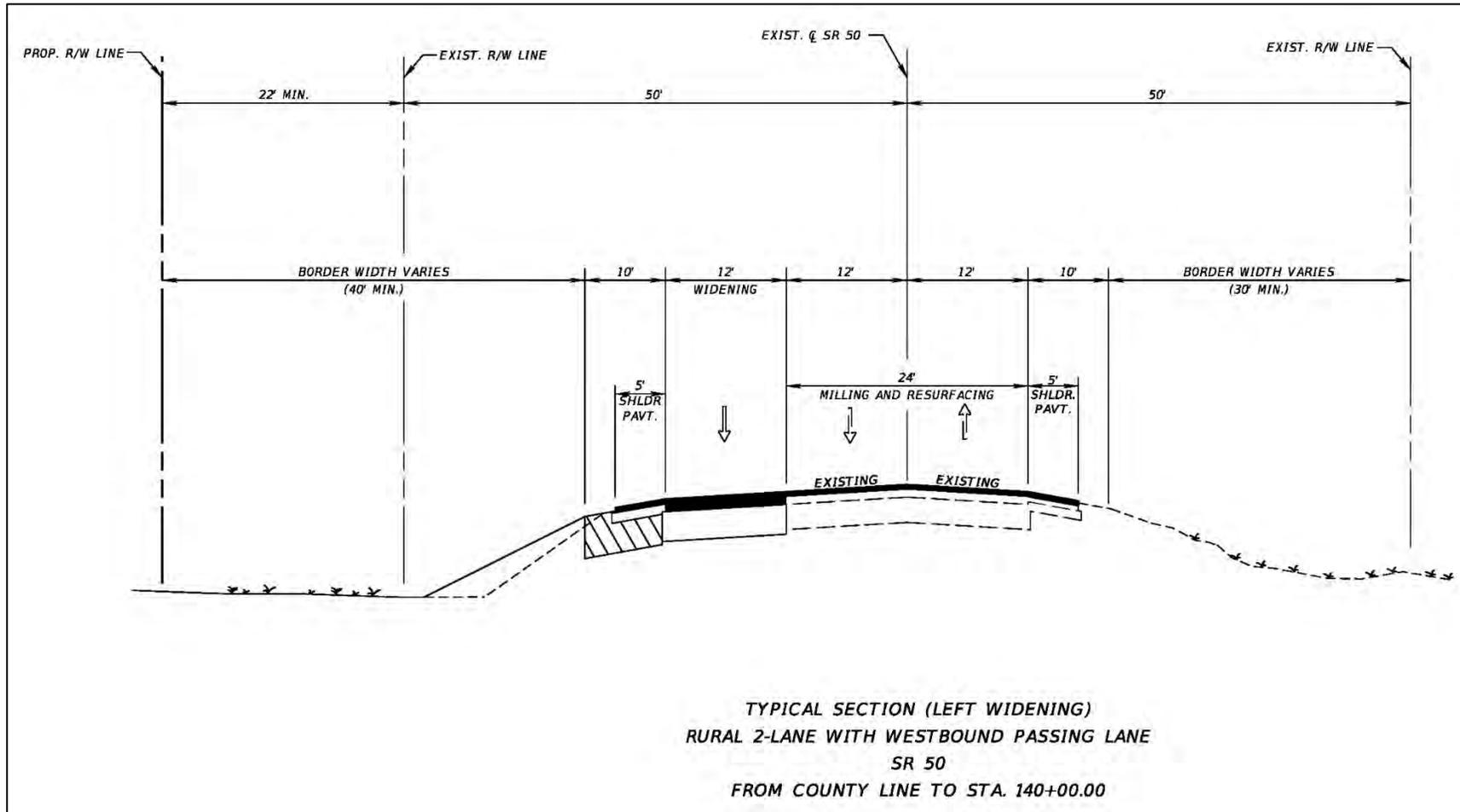
Figure 54: Westbound Passing Lane Center Widening – Station 2089+02 to Station 140+00
