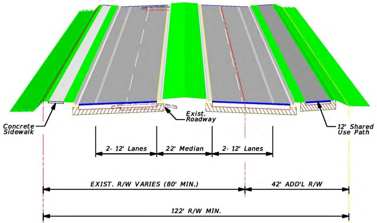
Figure 9: Typical Section – Lee Road to West of Barry Avenue (Maximum ROW with Drainage Conveyance Ditches)
