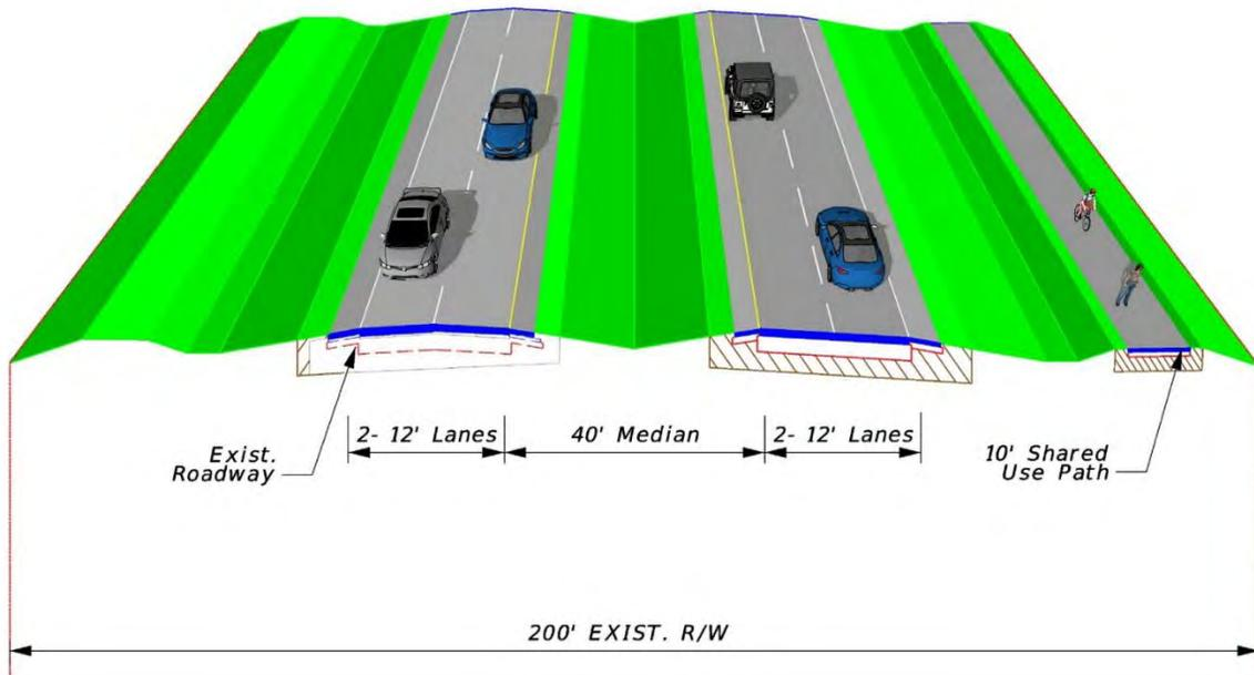
Figure 83: Typical Section – Railroad Overpass Bridges
