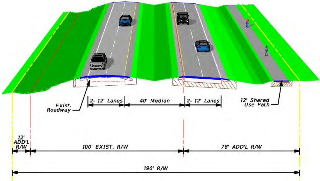
Figure 6: Typical Section – Hernando/Sumter County Line to Lee Road (Maximum ROW with New Construction and Drainage Conveyance Ditches)
