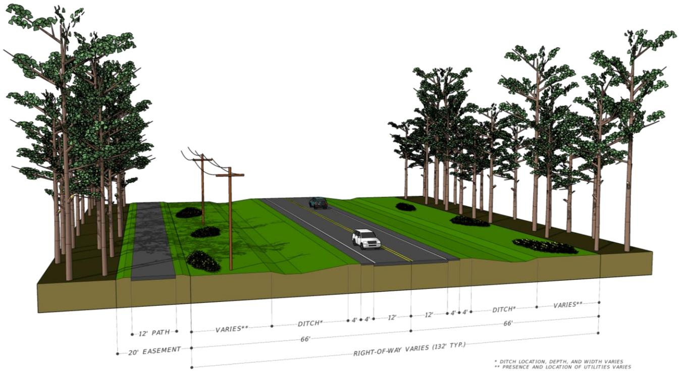
Figure 9 | Typical Section 3 – Constrained Areas
