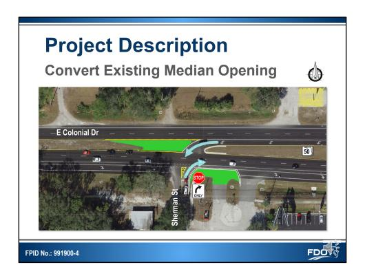
The proposed improvements at East Colonial Drive and Sherman Street consist of converting the full median opening to a directional opening. This means westbound traffic on East Colonial drive will still be able to turn left onto Sherman Street, but traffic leaving Sherman Street will be converted to right turn only.
