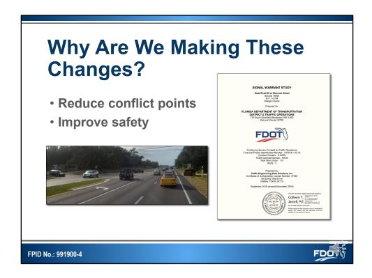
A Signal Warrant Study was conducted at this location in November of 2018. It was determined that a signal was not warranted, but it was recommended that the full median opening be converted to a directional opening to reduce the number of conflict points, which improves safety in the area.
