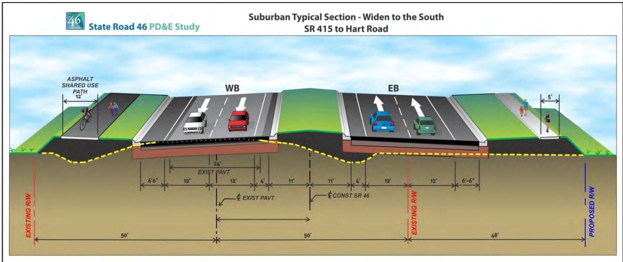
Figure 3: Proposed Typical Section (Segment 1)
