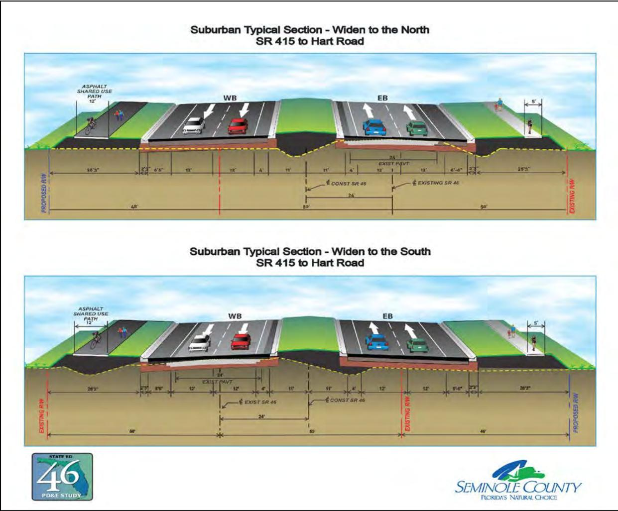
**Figure 5: Proposed Typical Section (Segment 3)**
