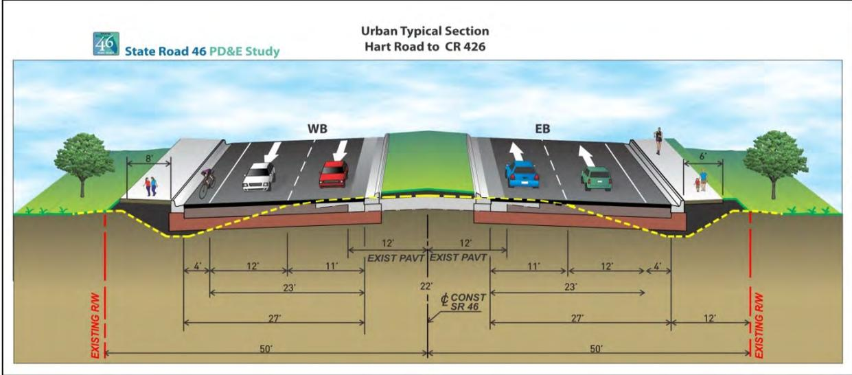
**Figure 6: Proposed Typical Section (Segment 4)**
