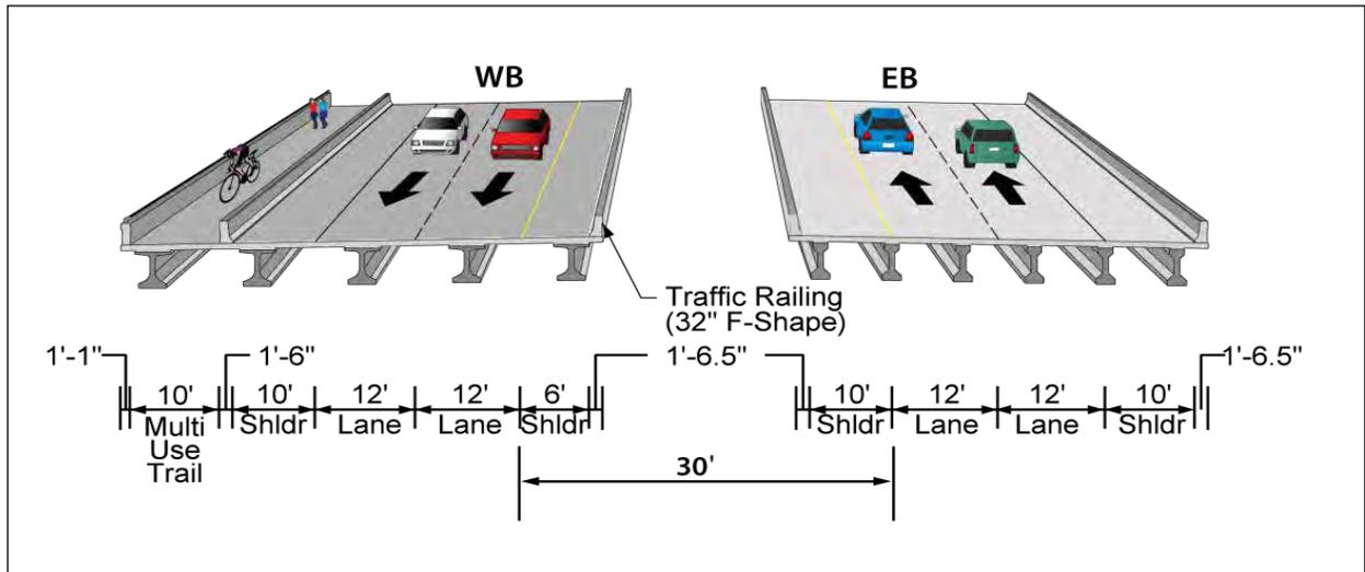
Figure 4: Proposed Typical Section (Segment 2)
