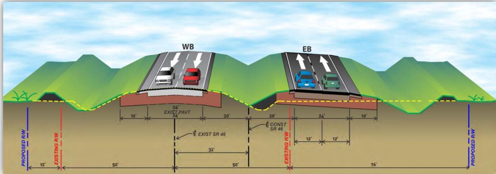
Figure 4.6 – Urban Typical Section – Centered Widening
