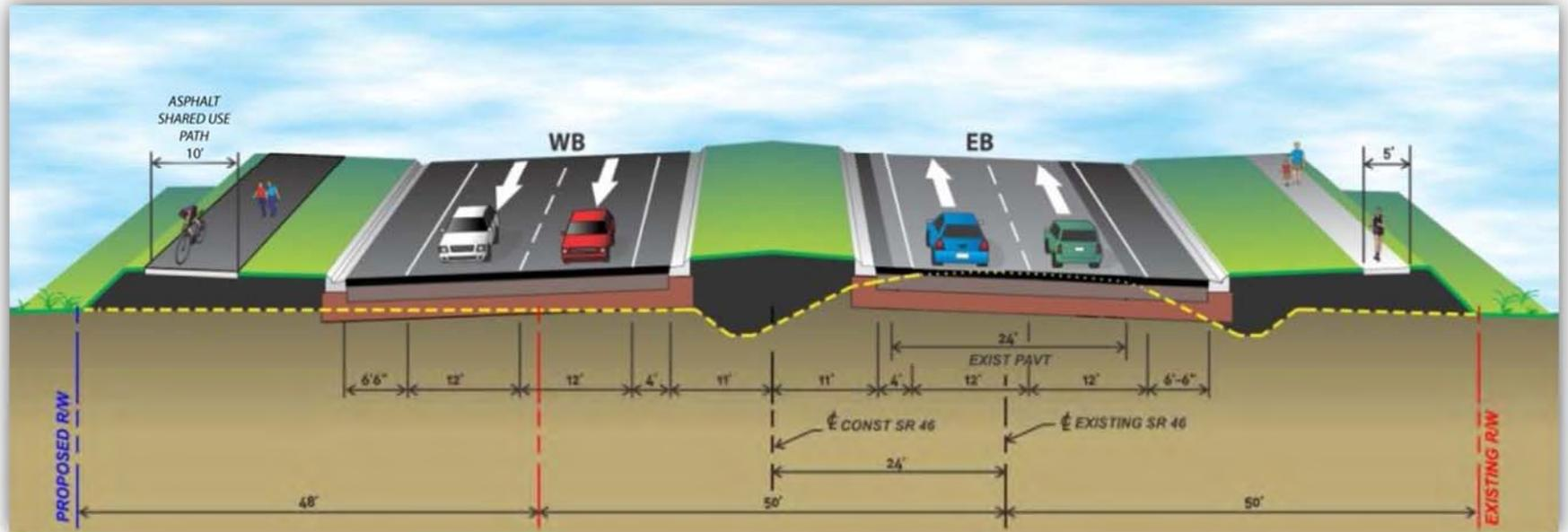
Figure 4.3 – Suburban Typical Section – Widen to the South
