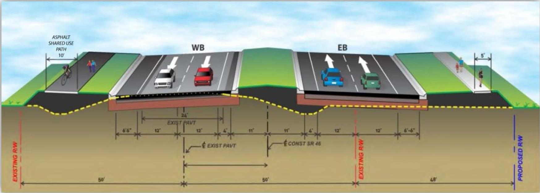
Figure 4.4 – Rural Typical Section – Widen to the North
