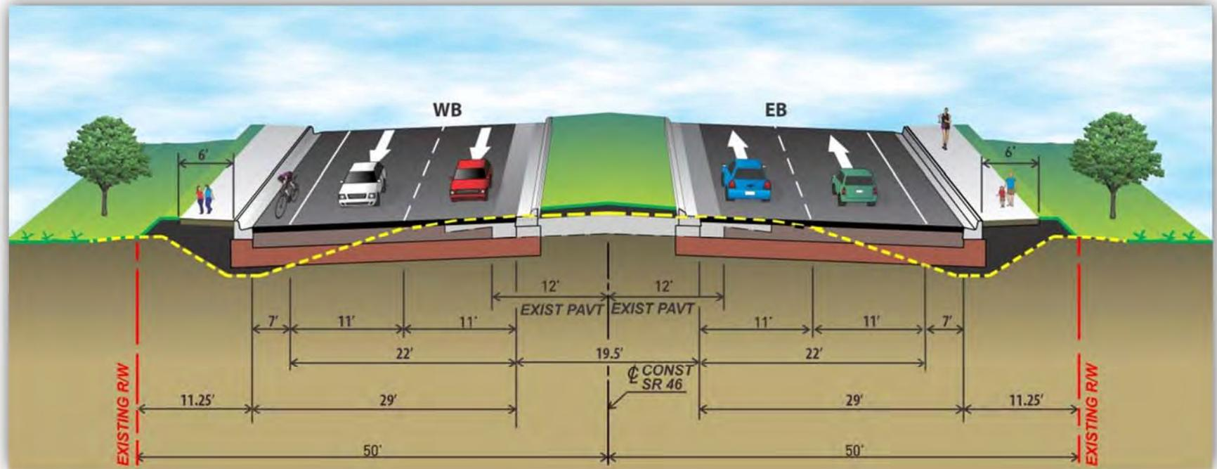
**Figure 4.8 – Bridge Typical Section without Shared Use Path**
