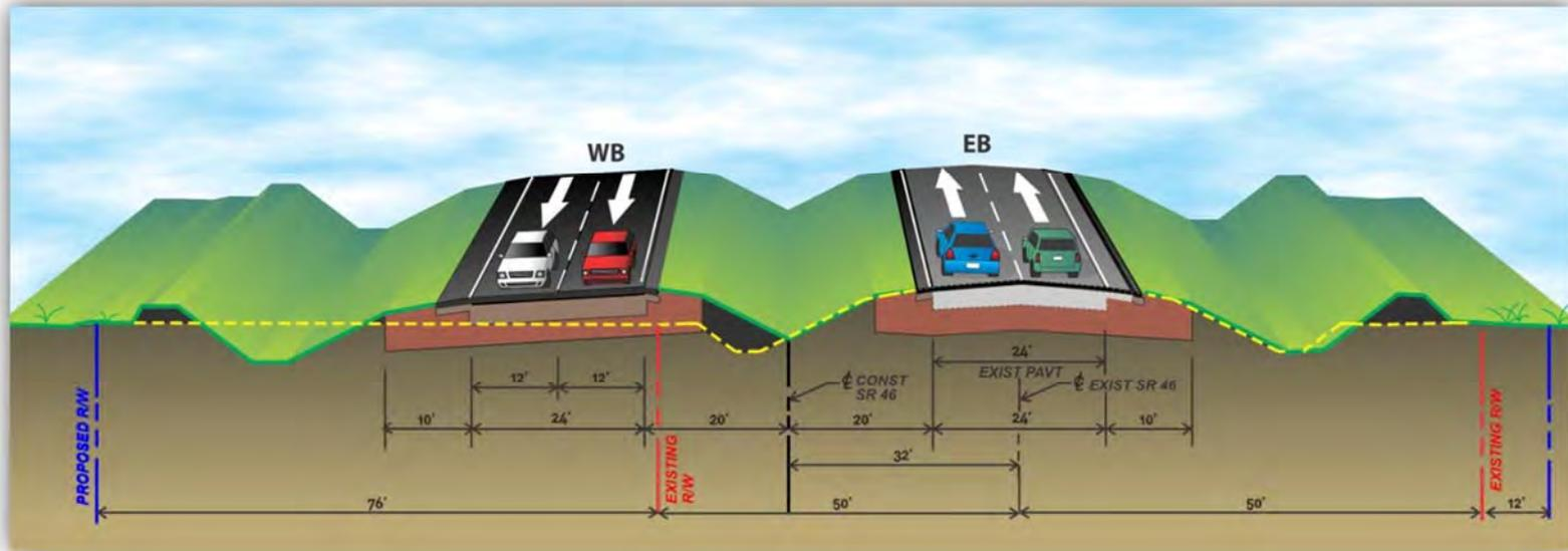
Figure 4.5 – Rural Typical Section – Widen to the South
