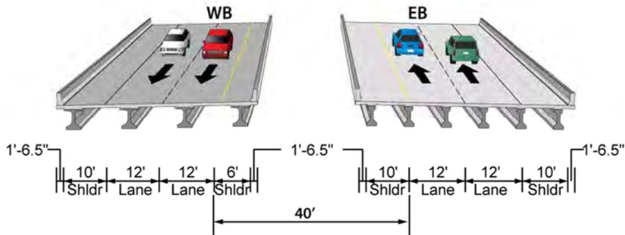
**Figure 4.9 – Bridge Typical Section with Shared Use Path**
