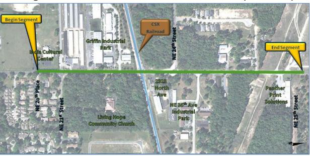
Shifting the alignment about 40 feet to the east in Segment 2 (south of the CSX rail line) eliminates the need for additional right-of-way from three parcels on the west side of NE 36<sup>th</sup> Avenue. This shift also reduces impacts on the overhead power lines that are located on the west side of the roadway. Right-of-way acquisition is funded in Fiscal Year 2017 and construction is funded in Fiscal Year 2019.
