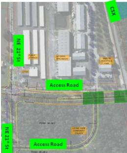
The shift to the east changes the Texas U-turn area by: allowing the existing NE 36<sup>th</sup> Avenue roadway to be used during the construction of the bridges, providing better driver visibility, improving the access road alignment, and a more efficient retention pond layout.
