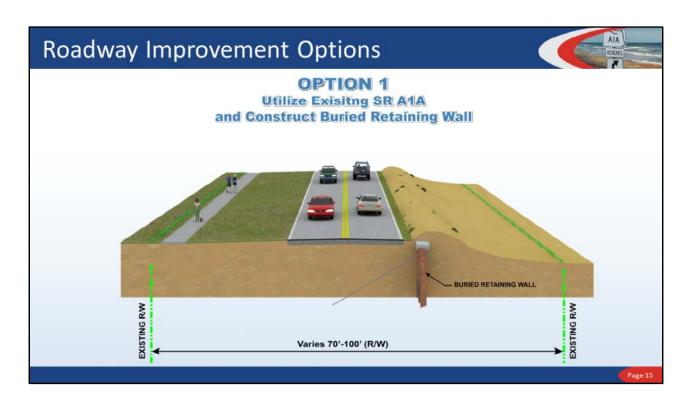
The first option would be to leave State Road A1A in its current location and construct a retaining wall that is covered with sand and native vegetation.
