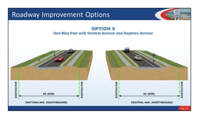
Option 5 would create one-way pairs using Central Avenue as the northbound lane and Daytona Avenue as the southbound. The existing State Road A1A would be removed and potentially replaced with a trail or other feature.
