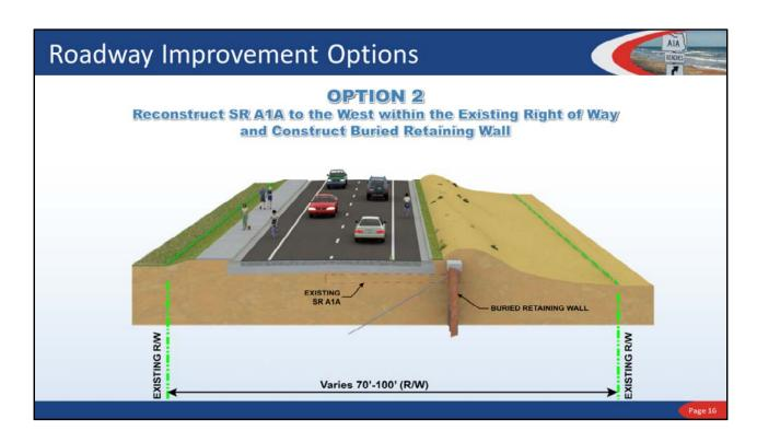
The second option would be re-construct State Road A1A as far to the west as possible within the existing right-of-way. A buried retaining wall would also be used in this option.
