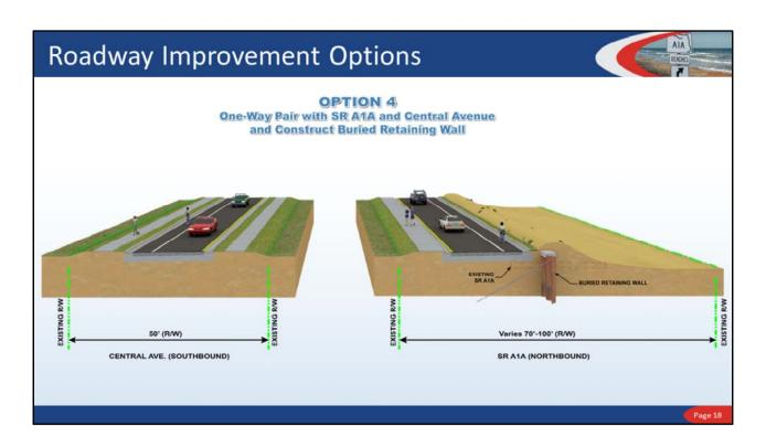
Option 4 involves creating one-way pairs using the existing State Road A1A right-of-way to construct the new northbound lane and converting Central Avenue to the southbound lane. This option also includes a buried retaining wall to protect the northbound lane.
