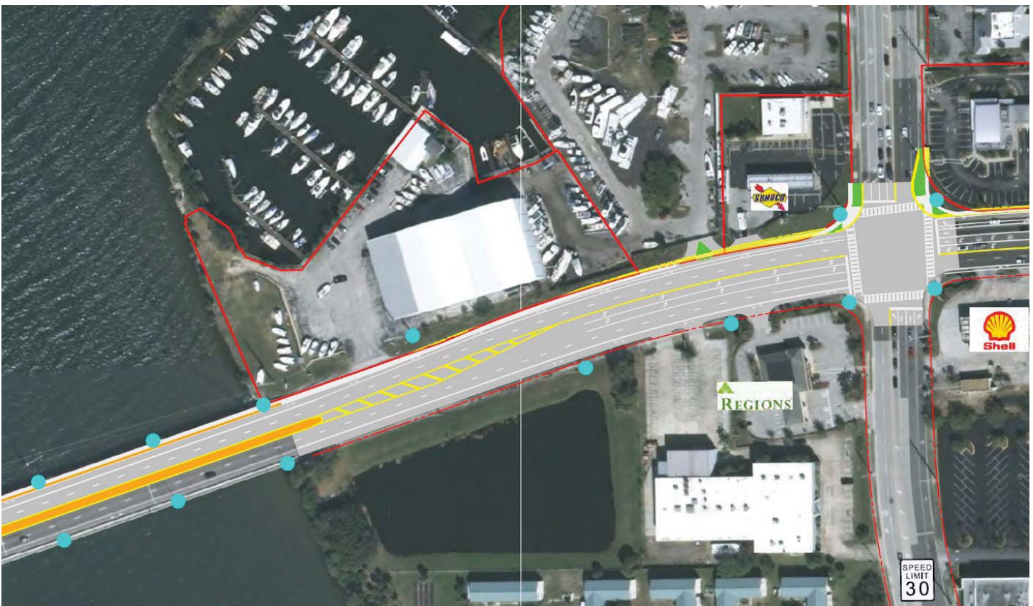
Exhibit 7: Plan View of Group 2 Improvements – Bulb out at South Patrick Drive, addition of separated sidewalk on bridge, lane realignment, sidewalks, bike lanes, and revised laneage
