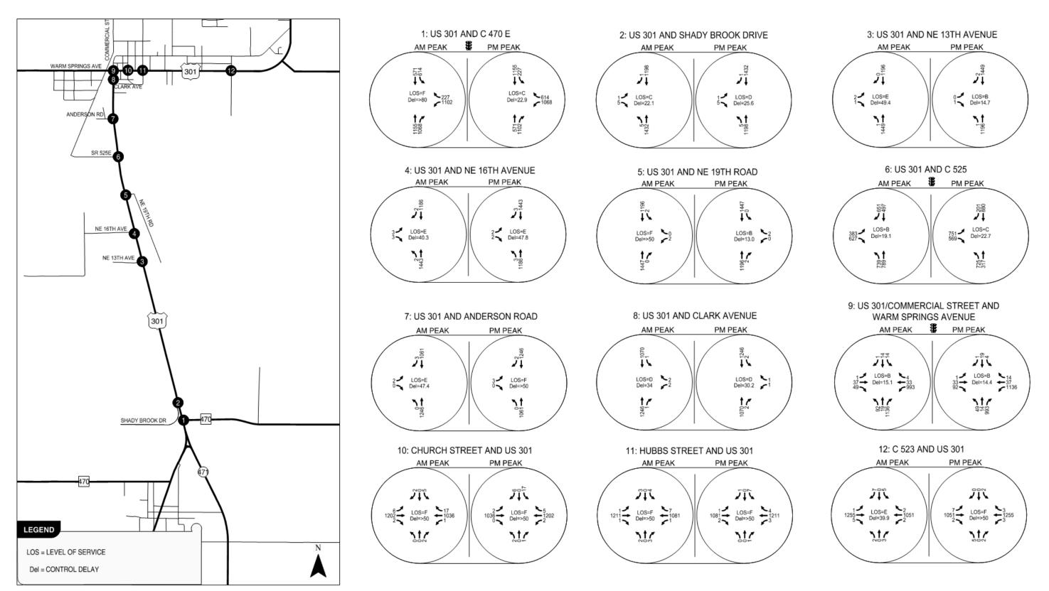
Figure 4-14 | 2042 Alternative 1 – AM/PM Peak-Hour Volumes and LOS – Part B
