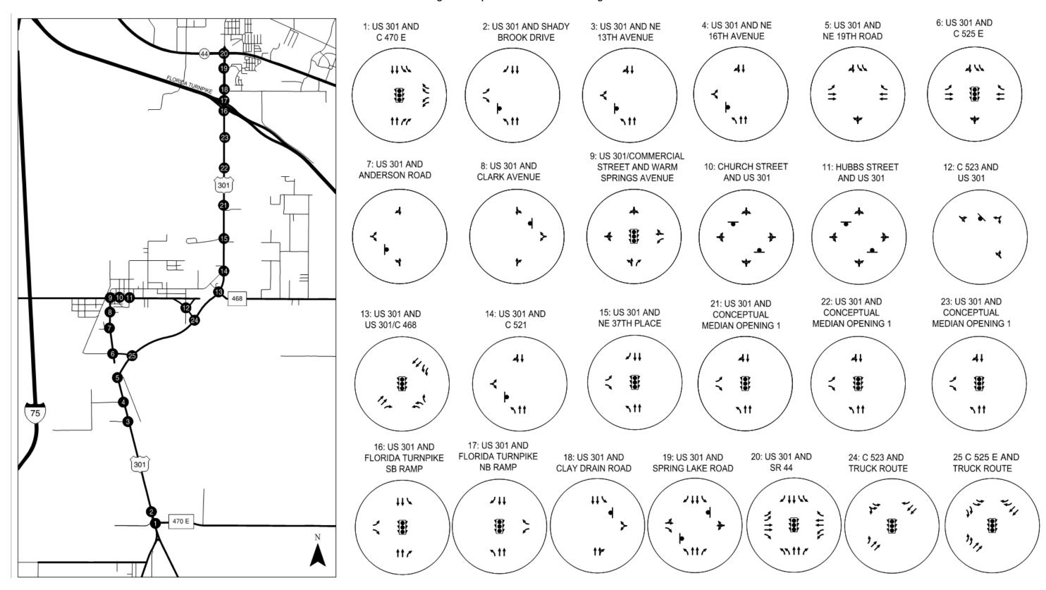
Figure 4-16 | 2042 Alternative 2 – AM/PM Peak-Hour Volumes and LOS – Part A
