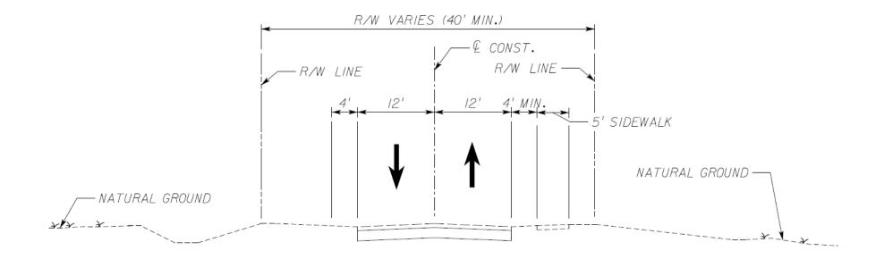
Figure 2-5 | Existing Typical Section – Segment 3 (Commercial Street to Stokes Street)
