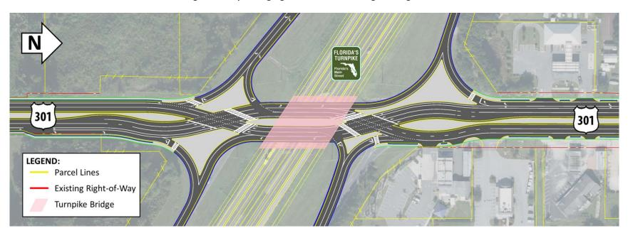
Figure 4-24 | Diverging Diamond Interchange Configuration
