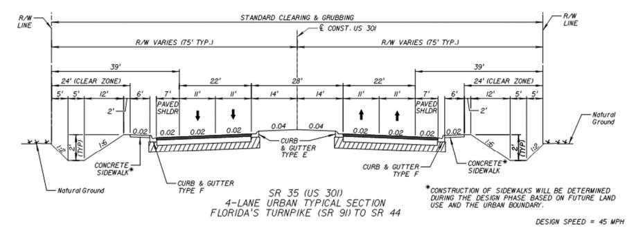
Figure 1-4 | Recommended Urban Typical Section – Segment 5
