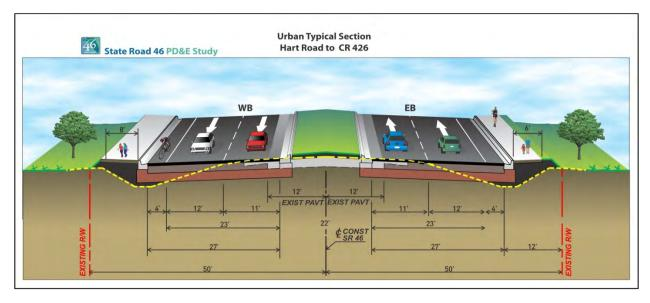
Figure 6: Proposed Typical Section (Segment 4)
