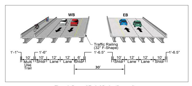
**Figure 4: Proposed Typical Section (Segment 2)**
