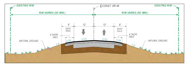
Figure 2: Existing Typical Section
