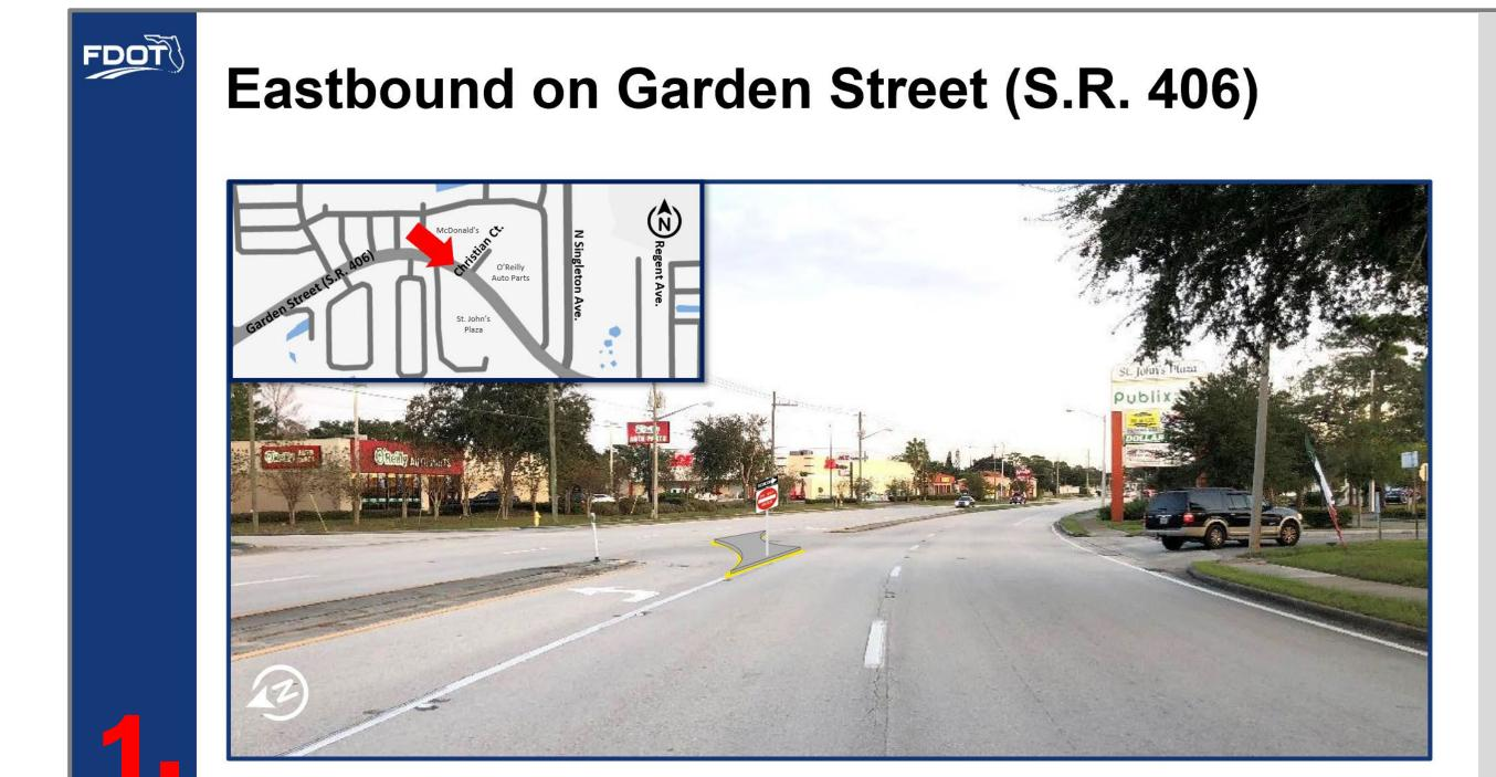
Proposed improvements eastbound on Garden Street (S.R. 406), including the construction of a median island, creating a bidirectional median opening.
