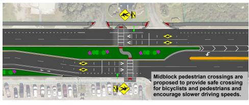
crossing will be equipped with Rectangular Rapid Flashing Beacons (RRFBs) or Pedestrian Hybrid Beacons (PHBs). These pedestrian activated lights make the crossings more visible and safer.
