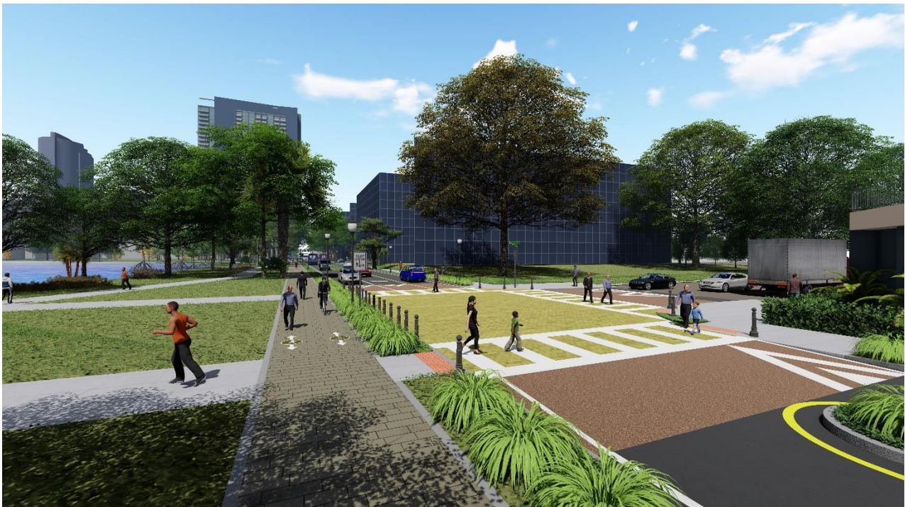
Raised intersection and crossing at Robinson Street and Broadway Avenue
