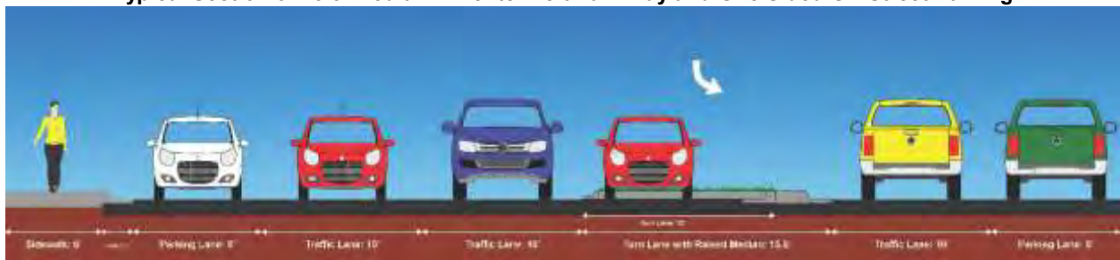
Typical Section 5: 15.5' Median w/Center Left Turn Bay and One Sided On-Street Parking
