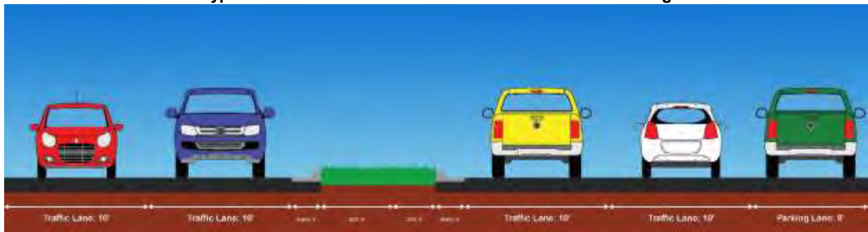
Typical Section 4: 8' Median w/One Sided On-Street Parking
