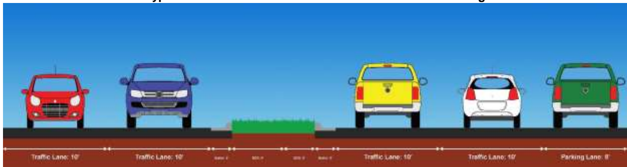
Typical Section 4: 8' Median w/One Sided On-Street Parking
